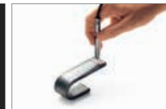
Ferrite content measurement in the weld seam area
