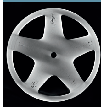
Cone-beam CT without BHC
