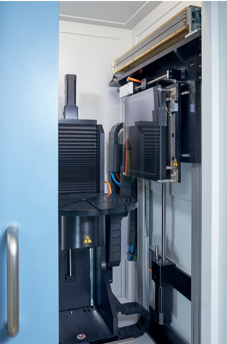
Configuration with line- and flat-panel detector
