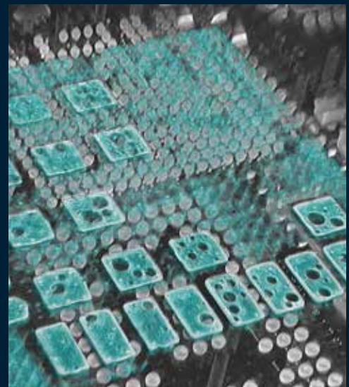
Computed Laminography of PCB, Clipping Plane
