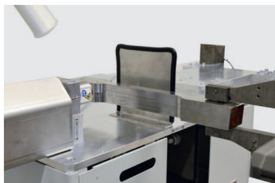
Specimen marking in the automated test centre
