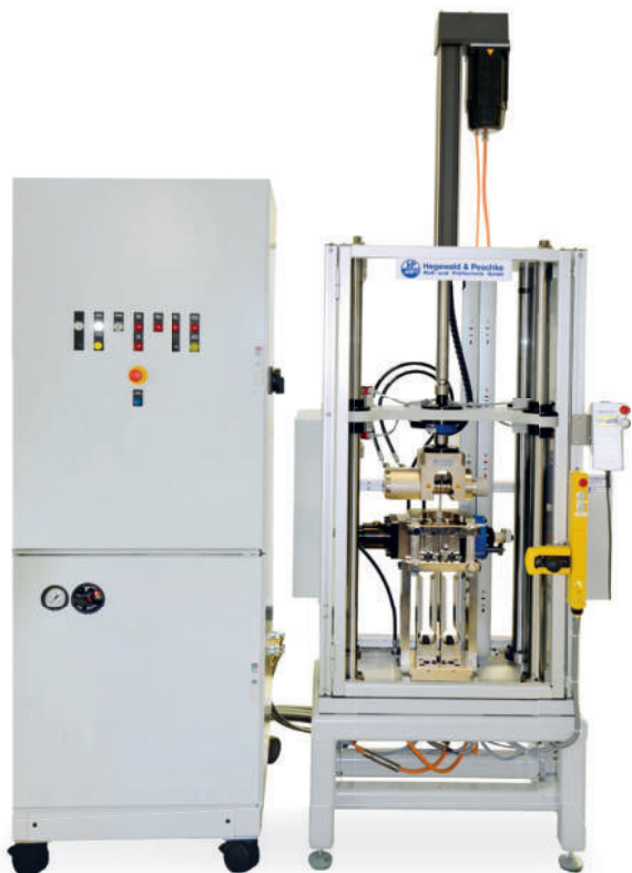
Special purpose machine for the draw bead test on body sheets
