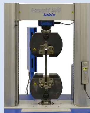
Reinforcing steel testing with laser extensometer
