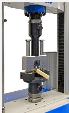
Shear test on wood ac- cording to DIN 52187
