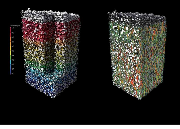
Color-coded visualization of transport phenomena, left: pressure, right: streamline view
