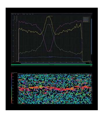
Top: Orientation tensor for the three main directions
