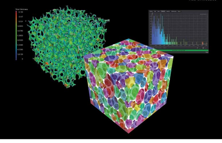
Visualize foam or foam-like structures and calculate properties
