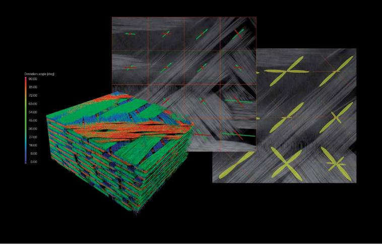
Analyze fiber composites, color code different fiber orientations, see main directions, and display orientation distributions
