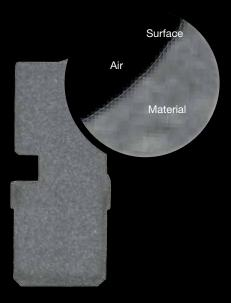
The surface is between material and air. Often, the surface is defined by a single gray value. When using Advanced Surface Determination, however, the gray values are processed depending on the gray values of the surrounding voxels. The result is a much more accurate surface.
