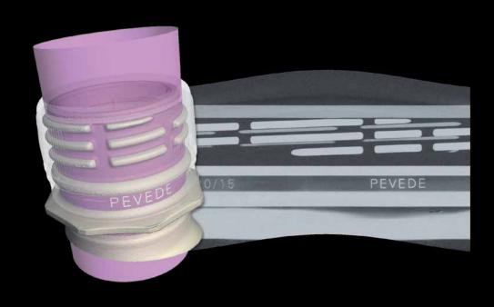
The cylindrical surface of a bottleneck has been unrolled to be viewed in a 'flattened' slice image.
