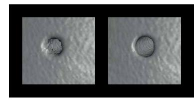
Not just smoother but also more accurate: Using the subvoxelaccurate surface determination (right) reduces your measurement uncertainty by giving you details the voxel-based surface determination (left) is not able to show.
