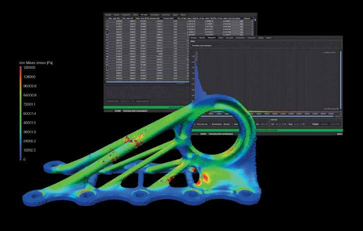
Color-coded display of the locations of the weak points directly on the scan of an additively manufactured cabin bracket
