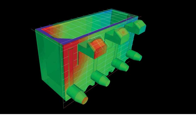
Get a color-coded visualization that shows you at a glance any deviations of the manufactured part from the target model.
