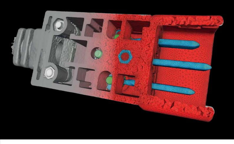
The Volume Meshing Module generates high-quality, solver-ready meshes.
