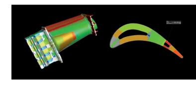
Color-coded results of a wall thickness analysis
