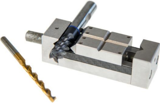
*Using special holders, it is possible to reliably measure even samples with complex shapes*
