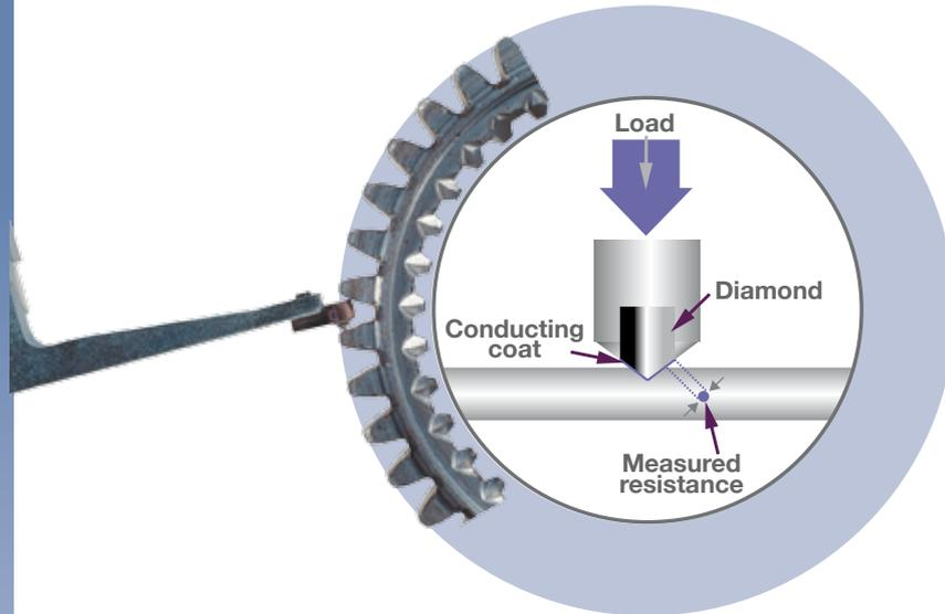
The diamond indenter can be compared to a little potentiometer, which, while gradually pushed into the material, obtains all the data (load-hardness) during the whole phase of load application.
