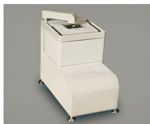
Polishing & Etching Unit
