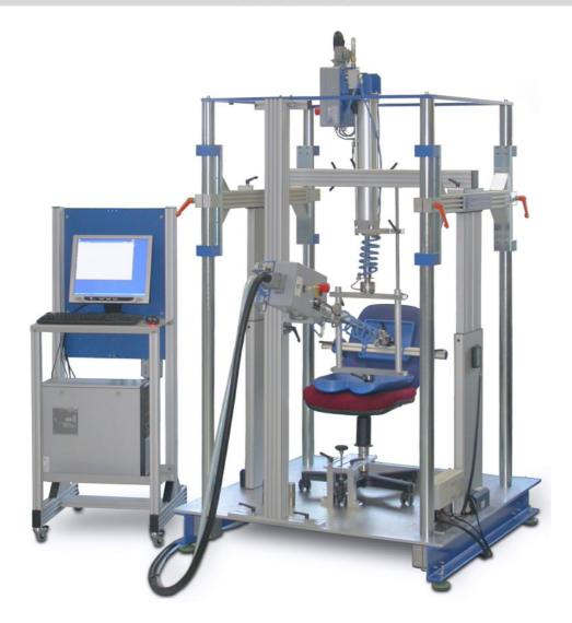
Test rig for alternating bending tests of seat and backrest according to EN 1335, EN 581-2-3, EN 1728, DIN 68878, BIFMA X5.1, NEN 1812, load or load/position controlled.
