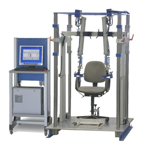
Test rig for alternating bending tests of arm rests according to EN 1335, EN 581-2-3, EN 1728, BIFMA X5.1, DIN 68878, NEN 1812, load or load/position controlled.
