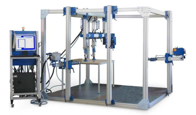
The universal testing rig is designed for testing seating furniture, tables, and upholstery acc. to EN 527-3, EN 581-2-3, EN 1728, EN 1730, EN 1335, BS 5459, BIFMA X5.1, as well as other current national and international standards. It includes 4 pneumatic test axes, load pads, load cells, and extensive testing and evaluation software.
