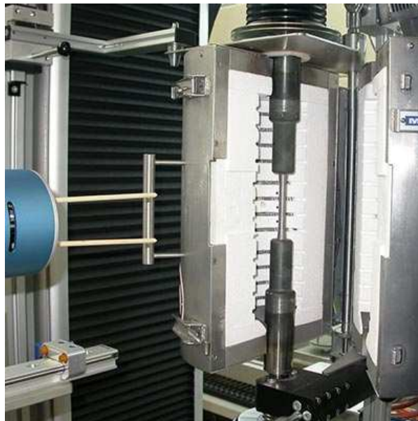
High-temperature kiln with extensometer installed in a universal testing machine
