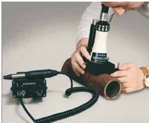
MOBISCOPE Portable Microscope
