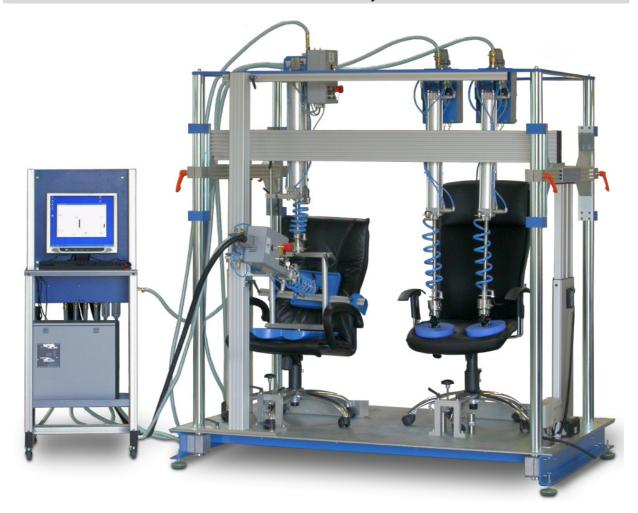
Double test rig for alternate bending tests seat, backrest and Side-to-Side tests according to EN 1335, EN 581-2-3, EN 1728, DIN 68878, BIFMA X5.1, load or load/position controlled.
