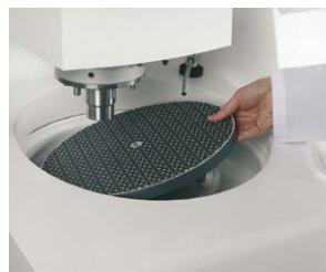
Simple exchange of working discs
