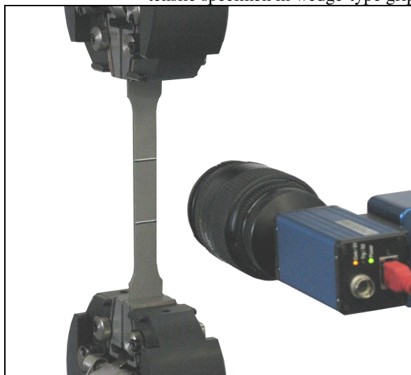
CCD camera with zoom-lens and tensile specimen in wedge-type grip
