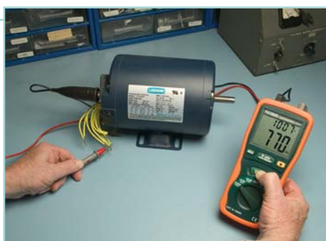
Measures the insulation resistance of motors.
