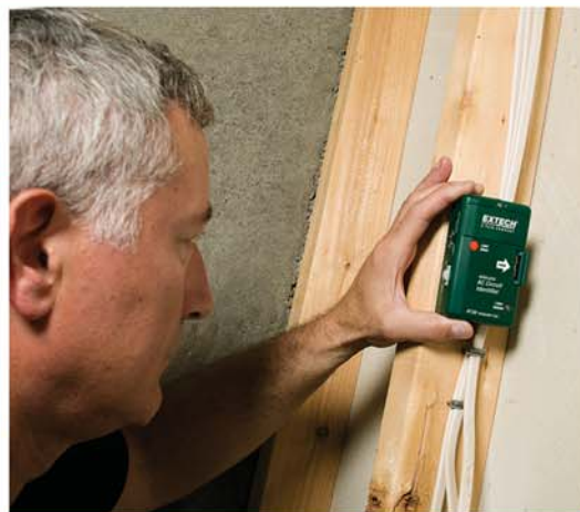
Wireless Circuit Detector for mid-run wires
