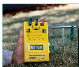
Check resistance between earth and grounding rod. Complete with test leads, auxiliary earth bars, heavy duty case, and six 1.5V AA batteries
