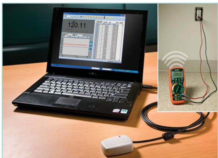
Continuous wireless data transmission from meter to your PC in real time
