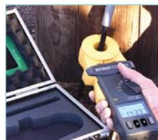
Verify resistance of cellular and communication tower ground grids
