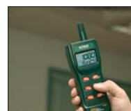
Measure CO 2 level in office buildings to check the air quality of conference rooms insuring proper ventilation.
