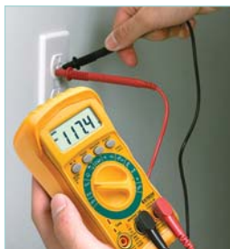
Model MN26T displays AC Voltage of an outlet receptacle using autoranging function.
