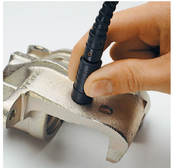
Measuring on rough surfaces, Zn/Fe with the ESD20Zn probe
