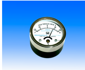
CALIBRATED FIELD INDICATOR Pt No 008M002 Scaled to +/- 20 gauss from zero for determining the level of residual magnetism to 5% of full-scale reading. Pt No 505056 As above except scaled to +/- 10 gauss
