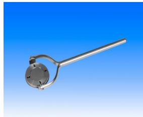
BERTHOLD PENETRATOR Pt No 008M006 Checks magnetisation, penetration depth, quality of fluorescent suspension and magnetic field direction
