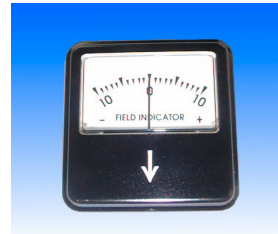
FIELD INDICATOR Pt No 008M001 Magnetometer used to determine if a component is magnetised
