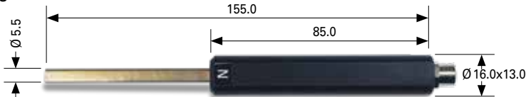
Flexible Reed Probe P-Z2/P-Z4: 0.9 mm thickness
