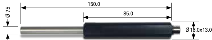
Tangential Field Probe P-T2/T4: 1.7 mm thickness
