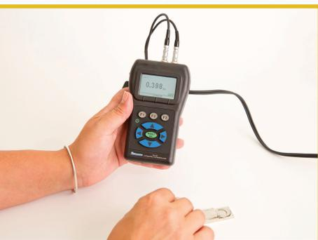
unprecedented measurements all at an entry level price. With the new Q-bar, even the most inexperienced operators can quickly determine if a thickness reading is stable. The EHC-03 offers a wide measurement range, two point calibration and even multiple on-screen languages. The EHC-03 is proudly made in the U.S.A. and has a 2 year warranty. Contact Danatronics for more details.
