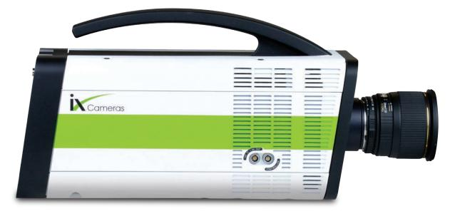
The i-SPEED 720 utilizes the same high-resolution 3 megapixel image sensor of the high-end i-SPEED 7 Series camera line, but at tempered speeds. Clocking at 20 gigapixels per second throughput, this camera can stop the world's fastest events. With internal memory options up to 144GB, the i-SPEED 720 is the ideal instrument for the test engineer, scientist or researcher.
