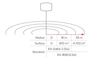
How to read the drawing: in a range of 39 m, being a surface of 4 700  $\mbox{m}^{2},$ we guarantee a lighting in accordance with the EN1838 standard.
