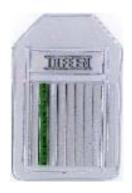
Wire type penetrameters, acc. to the European standard EN 462, 1994 issue. Number, arrangement, radius and material of each wire in this IQI correspond to the previous known DIN Image Quality Indicators (IQI) acc. to 54109, 1987 issue. Enclosed is certification of conformity for each BPK and the radiographic inscription at the top e.g. 10 FE EN. The letter "W" stand for "Wire". The thickest wire and with it the lowest Image Quality Class is W1.
