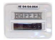
These IQIs consist of six steps with one or two holes of the same diameter as the thickness. The individual plaques are welded into a PVC pouch which also contains the lead identification. Each IQI is numbered and is supplied with a declaration of conformity within a storage wallet.
